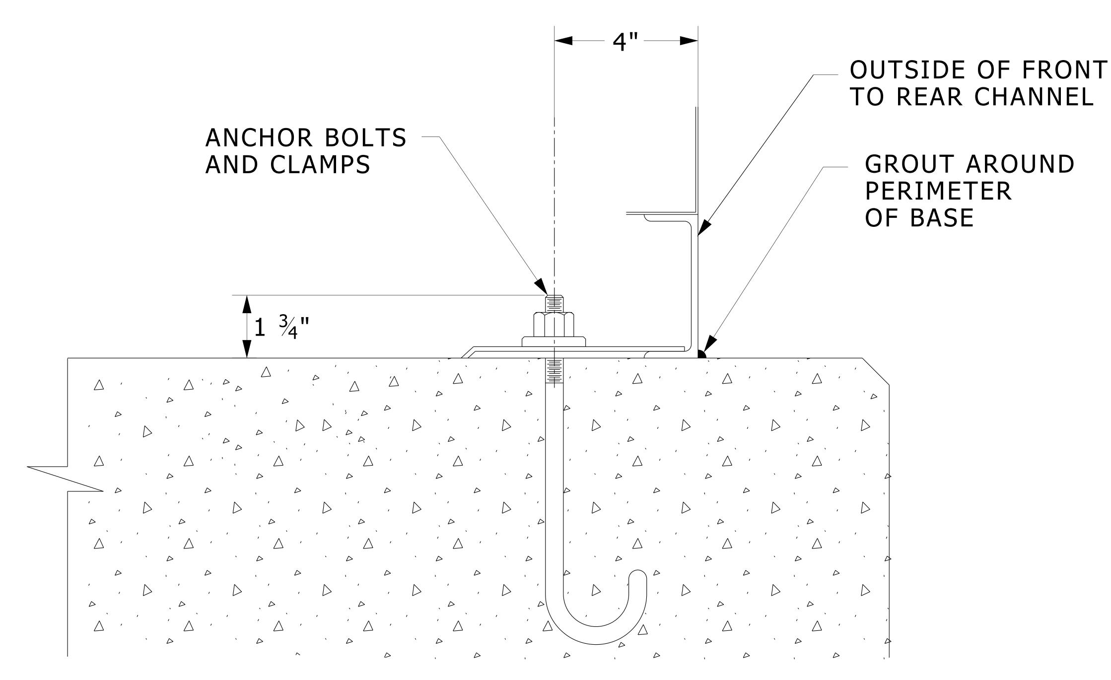
AFTER INSTALLATION OF SWITCHGEAR GROUT PERIMETER OF BASE ALONG LINE OF CONTACT WITH CONCRETE PAD. AND SEAL ALL CONDUIT ENTRIES,
